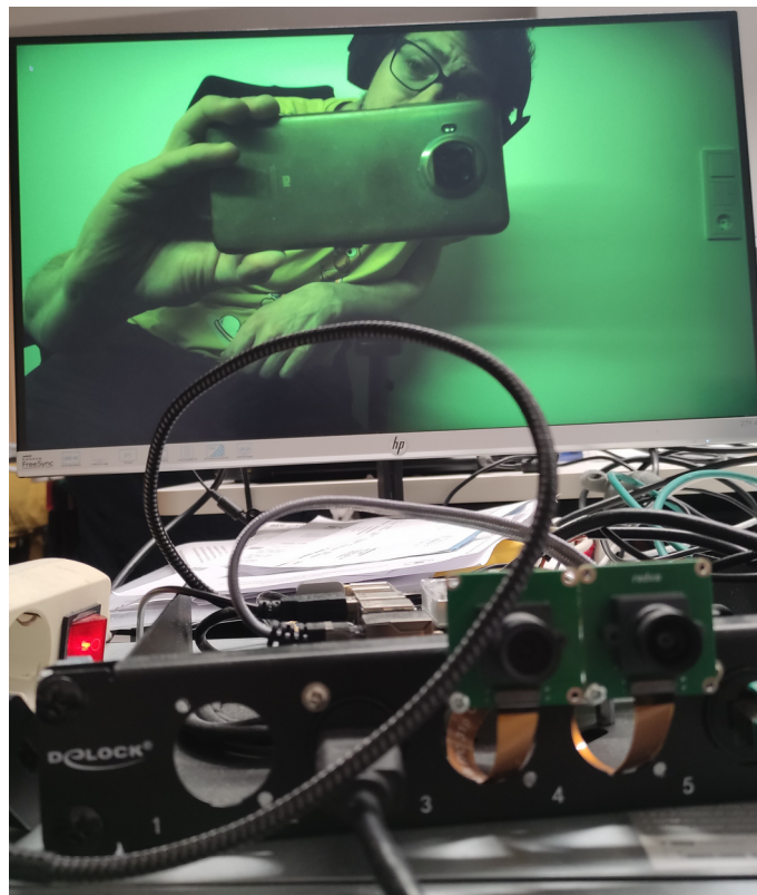
First stream with a Radxa ROCK 5B+ (RK3588) + Radxa Camera 4K (IMX415) via VICAP and ISP
